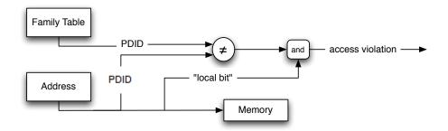
Figure 2: Implicit TLS protection mechanism
