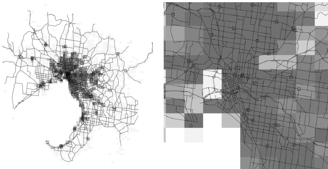
Figure 5. Road network, distribution of demand (darker regions correspond to greater demand), bases (squares), and hospitals (circles) in Melbourne.
