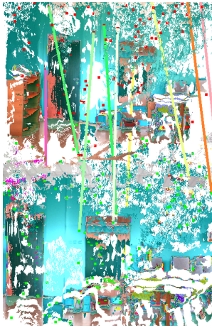
Fig. 4. Feature matching for coloured point cloud from stereo camera with Daisy algorithm
