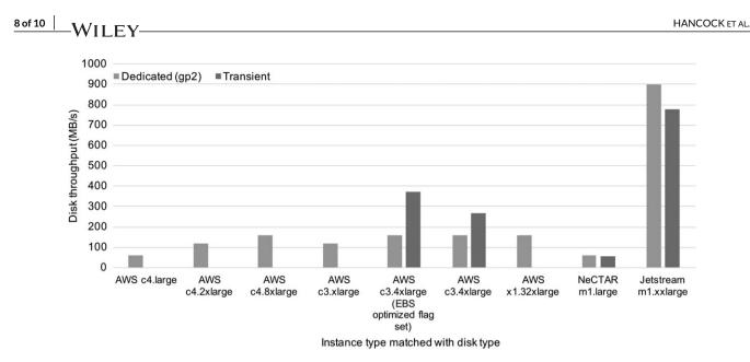
**FIGURE 1** Disk throughput performance using the fio command for a variety of disks and instance types from multiple cloud providers and shows the significant performance benefit of Jetstream resources
