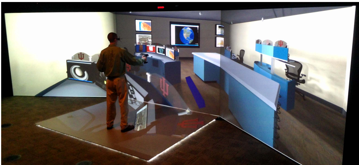
Figure 14. The IUPUI Virtual Reality Theater is a bright, high-resolution, immersive virtual reality technology suitable for individual and group use. The Theater is reconfigurable and driven by workstation computers running either Windows or Linux.
