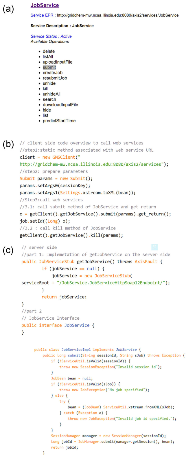
Fig. 5. Example of JobService web service. (a) JobService with its EPR and 14 operations. (b) Steps from Client-end to call JobService. (c) Server-end implementation of submit operation of JobService.
