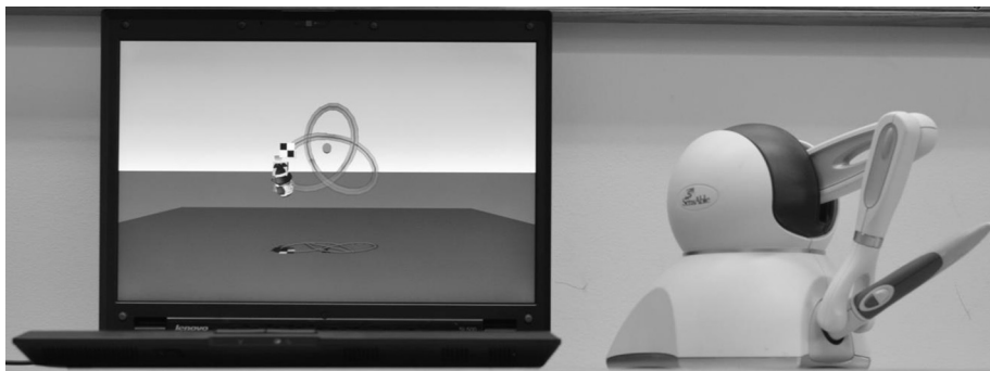
Fig. 1. An example display, showing a wire path, together with a Phantom Omni (Snapp-Childs, Casserly, et al., 2013).
