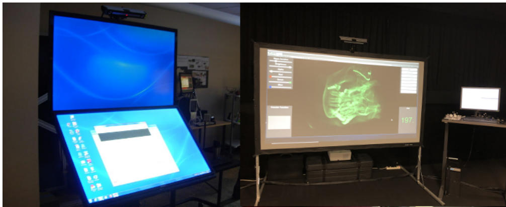
Figure 1: Examples of IQ-Stations. The left system with the lower touch display is deployed at University of Indiana’s Advanced Visualization Laboratory. The system on the right is deployed at Idaho National Laboratory’s Applied Visualization Laboratory showing a Unity 3D based volume renderer.
