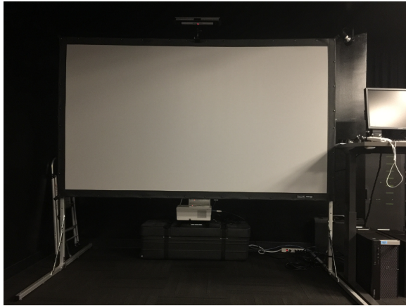
Figure 2: The short-throw rear projection IQ-Station utilizing the ART SMARTTRACK at INL.
