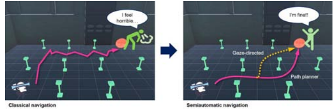
Figure 1: Left: with classical travel techniques, e.g., joystick-based techniques, irregular unsmooth trajectories lead to cybersickness. Right: with our semiautomatic travel technique, optimized smooth trajectories can be achieved thanks to automatic path generation, allowing reduced cybersickness.
