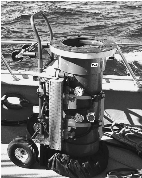
FIG. 3. Hyperbaric chamber set on end prior to receiving a fish. Secondary manifold is connected and visible on the left side of the chamber as viewed in the photograph.
