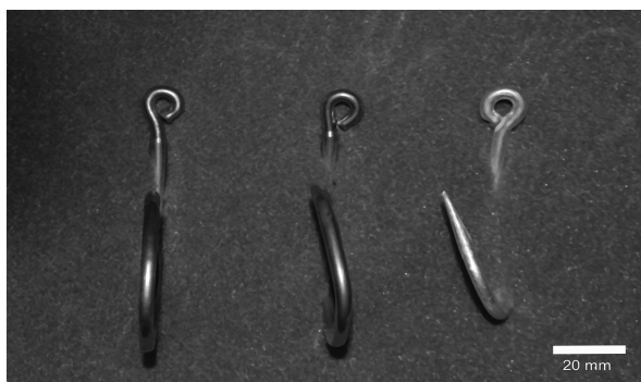
Figure 2. Hook offset ( 0^\circ , 10^\circ , and 20^\circ – 30^\circ ) as represented by a sampling of hooks models found in the data set, depicted from left to right: 18/0 0^\circ offset LP CIRBL; 18/0 10^\circ offset LPCIRBL; and 9/0 20^\circ – 30^\circ offset J-hook Mustad 76801 (no longer used by the US fleet).
