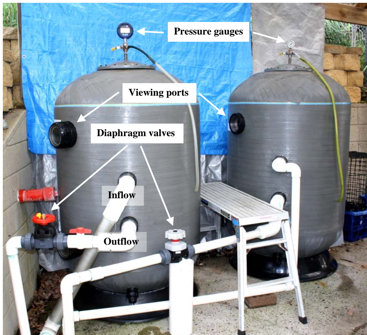
Figure 2.1. The twin custom-built hyperbaric chamber setup at the Cronulla Fisheries Research Centre of Excellence.
