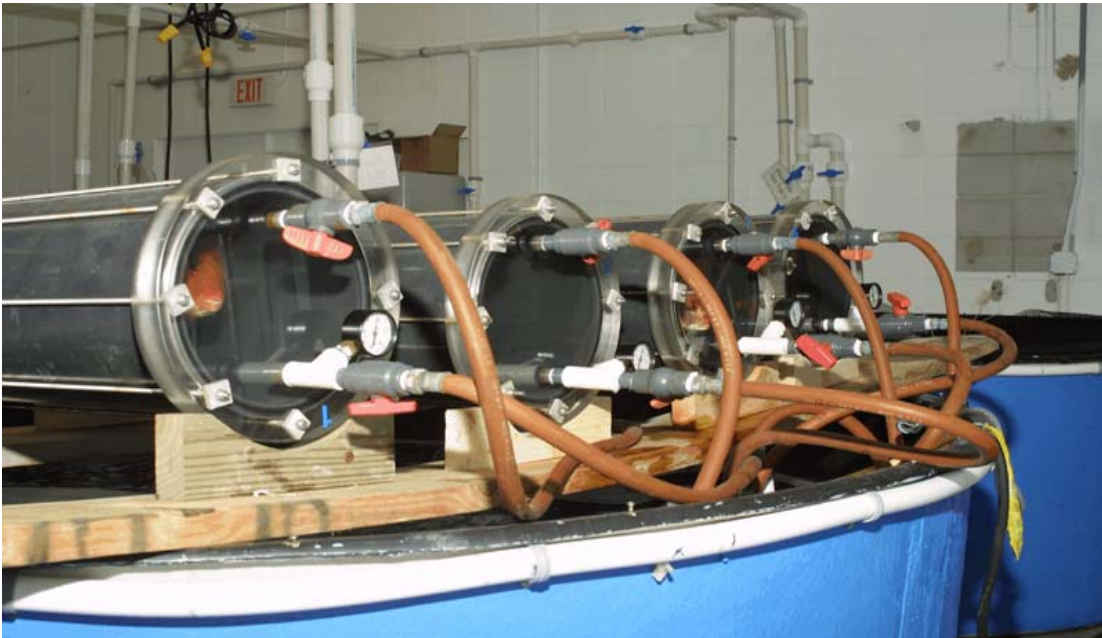
Figure 3. Series of fish hyperbaric pressure chambers situated over a 1,000 l tank, used in the pressure simulation experiments.
