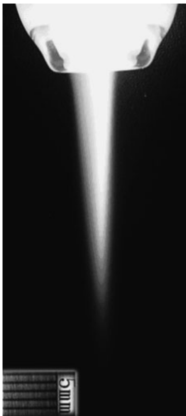
Figure 10. Photograph of the APGD plume developed by Chen et al. [34] The outer electrode is a solution of potassium chloride. The second electrode is a centrally located metal rod. The applied voltage is 30 kV at frequencies that range from 3 to 30 kHz.
