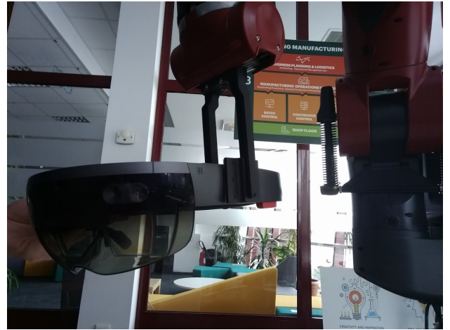
Fig. 6: Calibration procedure with Baxter and HoloLens
