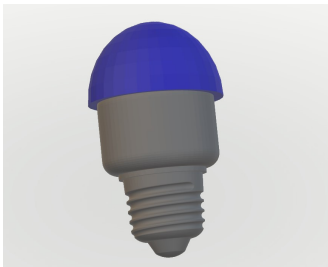
Fig. 5: CAD model with augmented part (blue)
