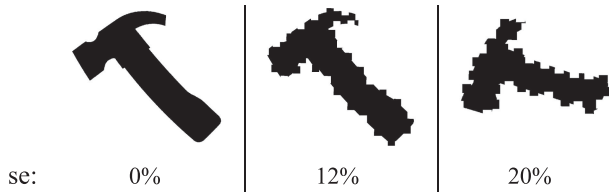
Fig. 2. Examples of various amount of segmentation errors ( se ). First an omnidirectional image without se , then the same test with se = 12\% , lastly the same template from a perspective test case with se = 20\% .
