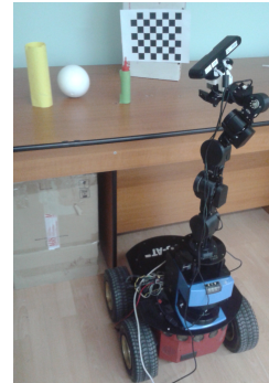
Fig. 1. The 7DoF robot arm model with the 3D depth sensor mounted on the top of it
