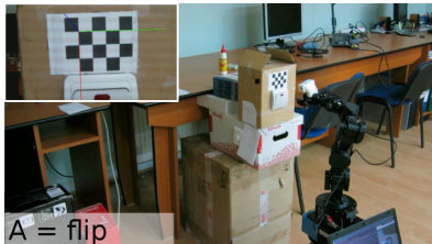
Fig. 8. Robot executing a flip action; the top-left inset is the camera view.
