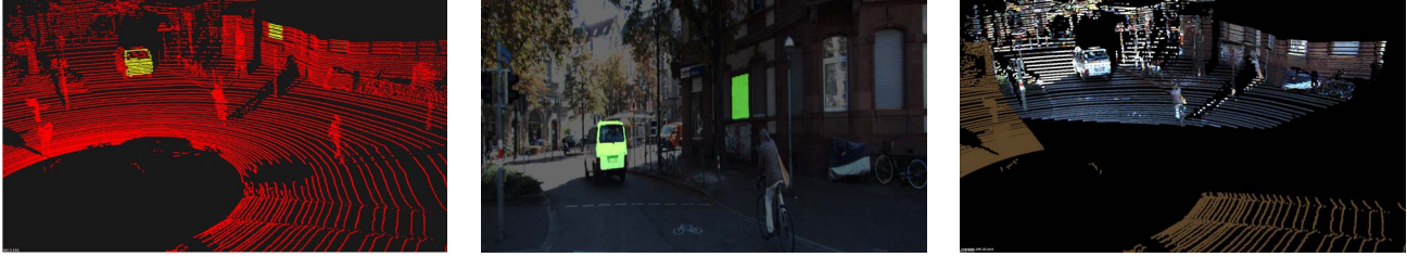
Figure 8. Calibration example with real data of an outdoor environment (left-right): 3D data with the selected region (yellow); color 2D data with the corresponding region (green); color information overlaid on 3D data using the extrinsic parameter estimates
