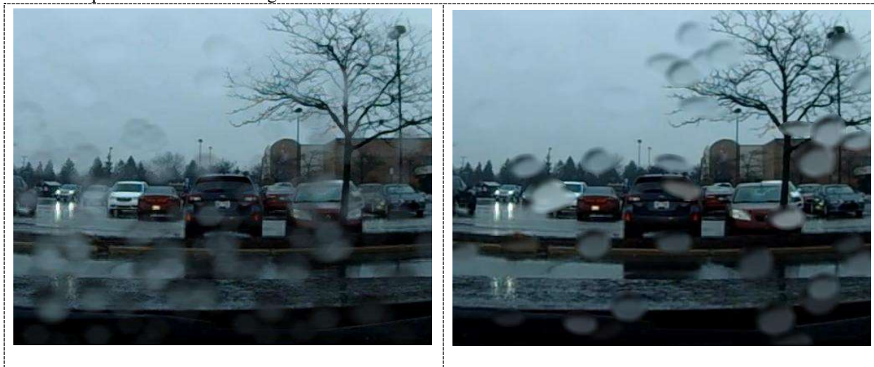
Figure 14: Images with raindrops that were generated by the ray-tracing method (left) and our method (right). Our model generates raindrops with more varieties in size, shape, and orientation compared to the ray-tracing model. The transparency levels in our generated raindrops are closer to that of real drops and are generally lower than that of raindrops generated by the ray-tracing model.
