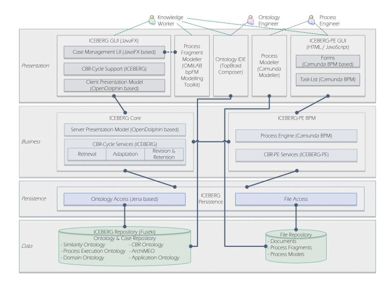
Figure 8.5: ICEBERG-PE System Architecture
