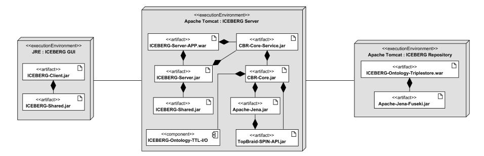
Figure 8.6: ICEBERG Deployment Diagram
