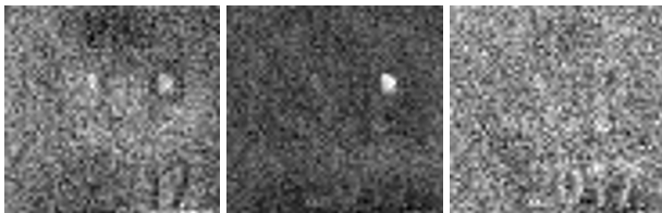
Figure 13: Residual image with subspace ranks of (left) five, (middle) eight, and (right) twelve. If the subspace rank is low, background and the anomalies have similar error. If rank is high, the residue is only noise, as the subspace captures anomalies as well. With a subspace of rank 8, the anomalous pixels within the letter “P” is clearly evident.
