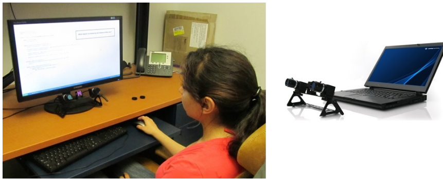
Figure 2: (Left) A participant sits in front of the computer and a video-based eye-tracker captures eye-movement data. (Right) FaceLAB is an example of video-based eye-trackers. This image is adapted from FaceLAB manual [54].
