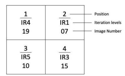
Fig.1: Left: 4-field-display area used for the 4-AFC test with the randomly selected CT images. Right: example of the assignment of the CT images randomly drawn for one particular permutation (combination 14 is shown). As described above, the numbers indicates the field position, the IR (i.e. the bins) and the number of the image.
