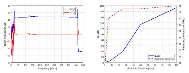
Fig. 3: Spectral response of (left) the Bloch impedance, and (right) the quality factor together with the resonance frequency as a function of the distance between the ZORA coil element and the overlying BTSL phantom.
