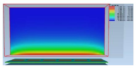
Fig. 2: Virtually uniform distribution of the transversal y-component of the magnetic field 10 mm inside the BTSL phantom.
