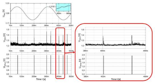
Fig. 2: left: Transient noise simulation of the presented recording channel, with the electrode voltage at the input stage  $U_{elec}$ , the output of the spike detection  $U_{EED}$  and the detected spike for the digital counter  $U_{APcnt}$  – right: Enlargement of the time period from 380 ms and 450 ms.
