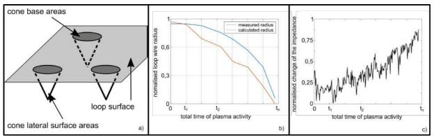
Fig.1: Model for diameter reduction (a)); Measured and calculated loop wire diameter (b)) and the resection electrode reactance (c)) in dependence of the total time of plasma activity
