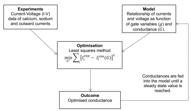
Fig.1: The flowchart of the optimisation scheme.
