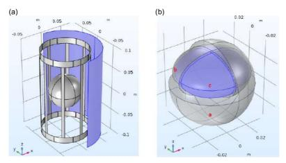
Fig. 1: (a) Birdcage coil geometry, EM shield and the phantom placed in the center of the coil. (b) Phantom geometry. The blue tissue (region c) is the brain tissue, region b is bone tissue equivalent and region a is filled with muscle.
