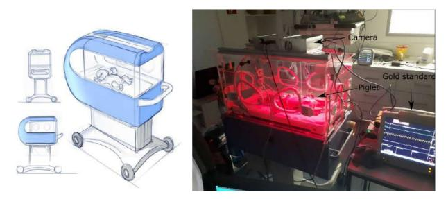
Fig.1: Left: Schematic representation of the project objective incubator. Right: Proof of Concept Incubator at a piglet measurement series at the University Hospital in Homburg.
