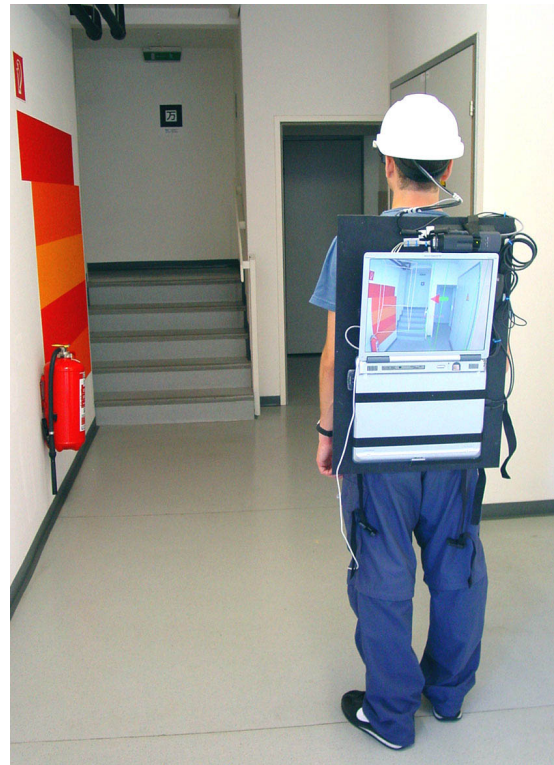
Figure 1: A user navigates through a building guided by the heads-up display graphics providing him with direction.
