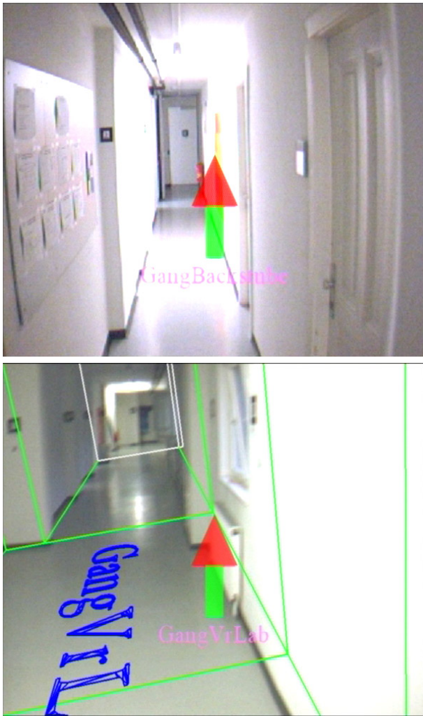
Figure 9: (Top) The direction is indicated by an overlaid arrow. (Bottom) The wire frame augmentation of the room and the portals can be switched on.
