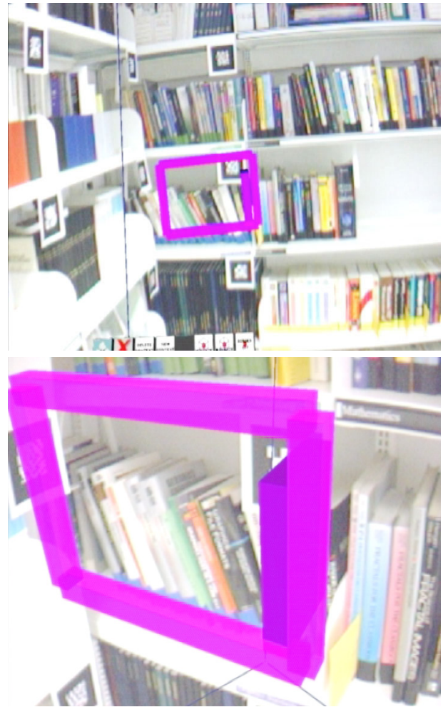
Figure 12: Augmented position of a book as seen by the user. These images were produced by overlaying the tracking camera's video image by the rendered graphics.
