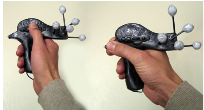
Figure 3: Eye of Ra - Input device for the hybrid user interface: The tip contains a conventional Tablet PC stylus tip for 2D interaction. Two buttons and a scroll wheel are used to trigger 3D interaction tasks. It is equipped with retro-reflective targets for optical tracking. The device is connected to the Tablet PC via a cable. Note the two different ways of grasping the device, the power grasp on the left and the precision grasp on the right.
