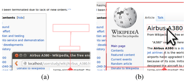
Figure 2: (a) Smart links pointing to out-of-viewport occurrences of a search term. (b) Hovering over a smart link reveals a semi-transparent overlay showing the actual content.
