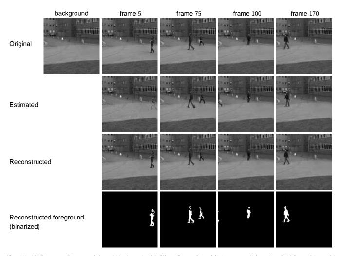
Figure 5. PETS sequence. The top panel shows the background and 4 different frames of the original sequence, which consists of 171 frames. The remaining panels show the estimated frames e[k], the reconstructed frame  $\hat{z}[k]$ , and the reconstructed foreground  $\hat{x}[k]$  (binarized for better visualization).
