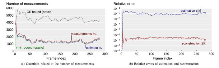
Figure 4. Results for the Hall sequence. (a) Number of measurements  $m_k$  taken from each frame (solid red line) and estimate  $\phi_k$  (dashed blue line); the dotted lines are the right-hand side of (6) and (7) (green and black, respectively). (b) Relative error of estimation  $\|e[k] - z[k]\|_2/\|z[k]\|_2$ , and reconstruction  $\|\hat{z}[k] - z[k]\|_2/\|z[k]\|_2$ . Figure (b) is illustrative, since the reconstruction error is mostly determined by the precision of the solver for (4).
