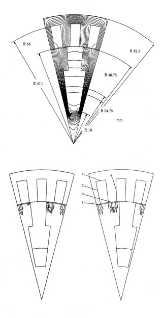
Fig. 3: Geometric data and some models with their surface force density
