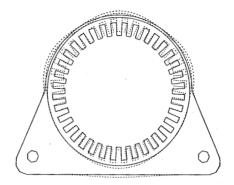
Fig. 11: Structure deformation - 24th harmonic - 7200Hz
