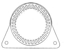
Fig. 10: Structure deformation - 16th harmonic - 4800Hz
