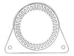
Fig. 9: Structure deformation - 24th harmonic - 3600 Hz
