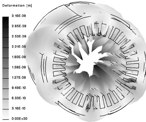
(b) Deformation of Stator.
