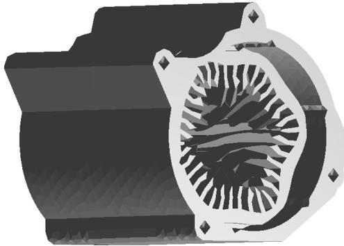
(a) Deformation of Stator and Casing.
