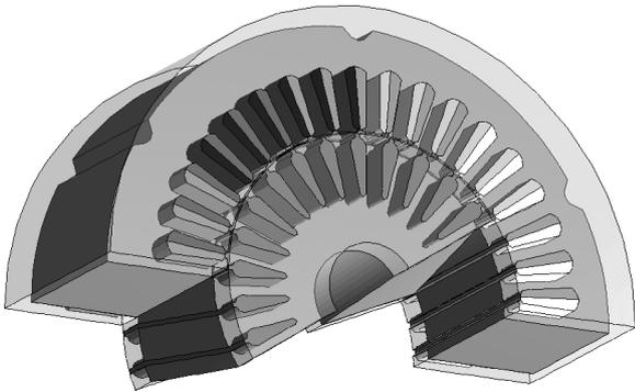
Figure 3: 3D FEM Model for Electromagnetic Simulation.
