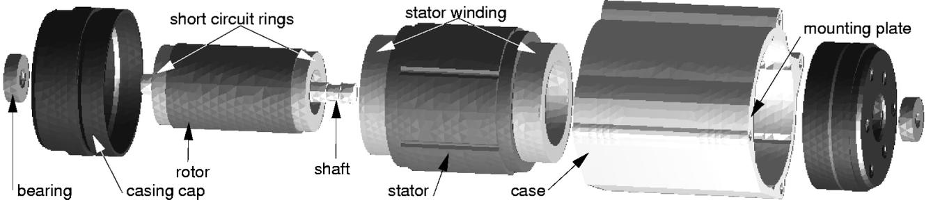
Figure 6: Exploded View of the Structure-Dynamic Model of the Induction Machine with Squirrel-Cage Rotor.
