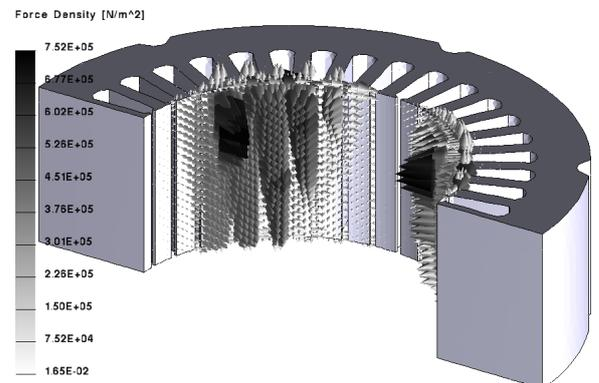
Figure 5: Surface-Force Density Distribution on the Stator Teeth for One Time Step (Only Stator Lamination Shown).
