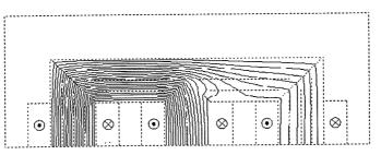
**Notes:** The phase of the currents in the coils is  $-85^{\circ}$ ,  $35^{\circ}$  and  $155^{\circ}$  respectively. The flux density in the middle limb is approximately alternating with an amplitude of  $1.17~\mathrm{T}$
