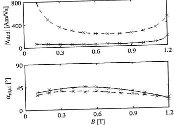
Figure 4. Reluctivity tensor entries  $|\nu_{\rm rd}|$  (top, solid),  $|\nu_{\rm td}|$  (top, dashed),  $\alpha_{\rm rd}$  (bottom, solid) and  $\alpha_{td}$  (bottom, dashed) as a function of the magnitude B of a circular flux density (Birkfeld, 1998)
