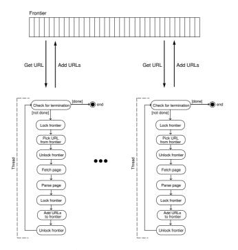
Fig. 3. A multi-threaded crawler model
