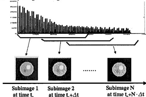
Figure 1. Sliding window reconstruction to get a set of subimages. However, since each of the subimages share some of the data (50% in this work) with the adjacent ones and the field map decay occurs during the acquisition, applying linear regressions to the phases of subimages introduces more error in the field map estimate than the standard two-point method. To reduce the error, an iterative method
