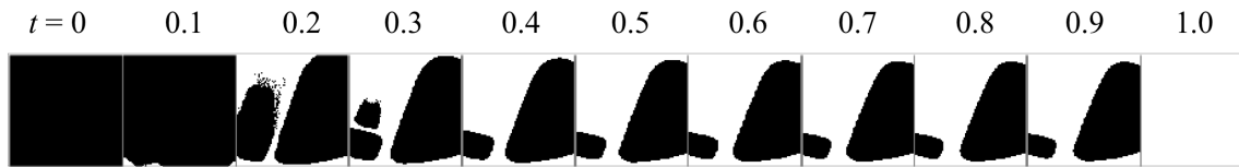
Fig. 27: Segmentation using threshold t = 0.1, 0.2, \dots 1.0 .
