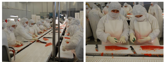
Figure 1. Typical manual operation in a processing line using pliers to remove fish bones in salmon fillets.
