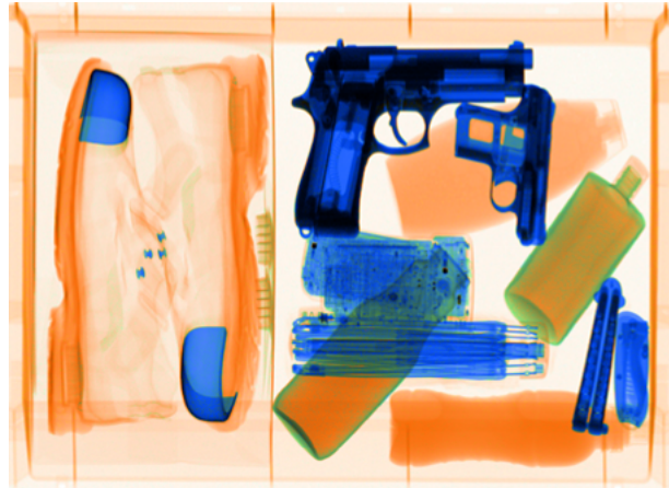
Figure 2. Generation of a pseudo-color image using dual-energy. In this example orange represents organic materials, and blue metals. The intensity of this image corresponds to the thickness of the materials (courtesy by M. Baştan [3]).
