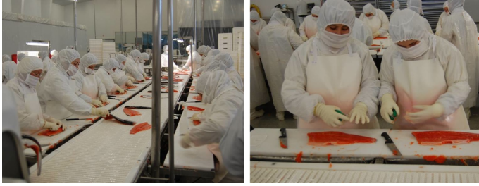
Figure 1: Typical human inspection in a processing line using pliers to remove fish bones in salmon fillets.
