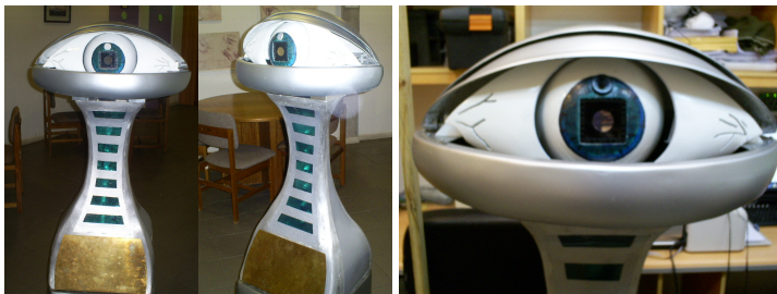
Fig. 10 a) Our social robot where its body correspond to a sculpture. b) The robot eye is its main emotional interface .
