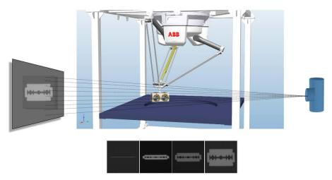
Figure 4: Schematic illustration of our X-ray system: the manipulator can locate the test object in different positions in order to analyze different projections.
