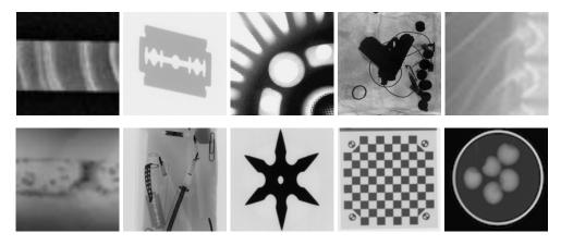
Figure 5: Some X-ray images of our public database GDXray: wood, razor blade, aluminum wheel, bag with a gun, fishbones, weld, pen case, shruriken, calibration pattern and apples.
