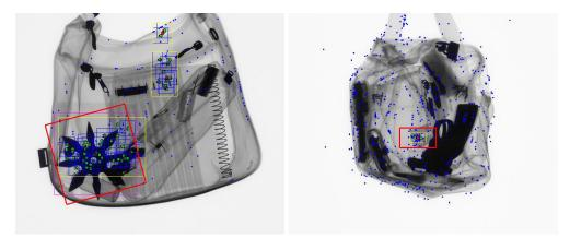
Figure 8: Detection of a shuriken (left) and a razor blade (right) using our approach based on ISM in a single view (see red parallelogram).
