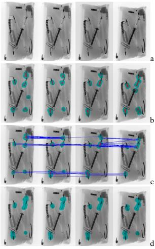
Figure 9: Multiple view detection of springs in a pencase: a) original test sequence, b) detected monocular keypoints, c) matched keypoints, and d) detection.
