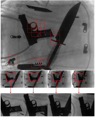
Figure 6: Detection of a gun in a bag. Top: single view detection of a gun, we observe that there are several false alarms. Middle: sequence with 4 X-ray images. Bottom: with multiple view analysis false alarms are eliminated without discrimination of the gun.
