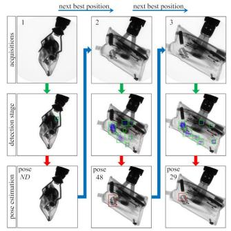
Figure 7: Detection of a razor blade in pencil case using active vision.
