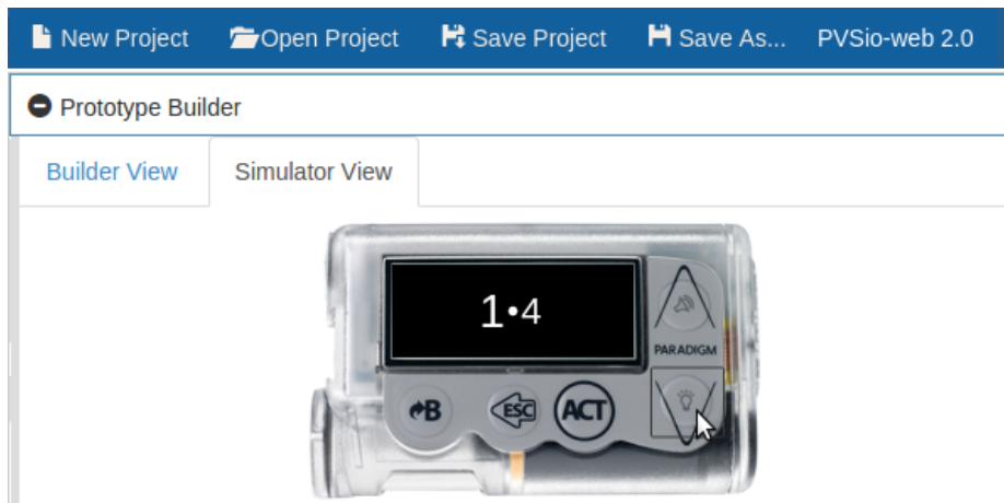
Fig. 4: The insulin pump prototype executed within PVSio-web.
