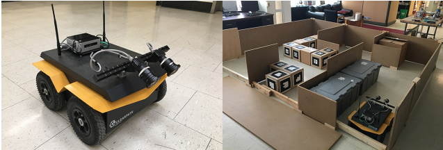
Figure 2: Clearpath Jackal UGV robot used for real-world experiments.
