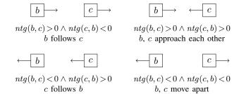
Figure 1: The sign of NTG indicates the driving direction: ntg(b,c) is positive iff b moves towards c's position.
