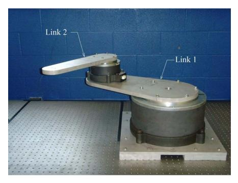
Figure 4-1. The experimental testbed consists of a two-link robot. The links are mounted on two NSK direct-drive switched reluctance motors.
