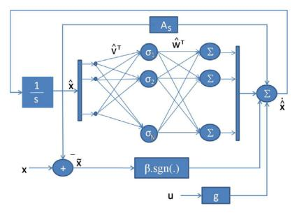
Figure 3-1. The architecture of the MLDNN.
