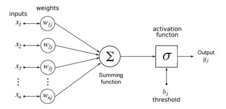
Figure 2-1. Nonlinear model of a neuron
