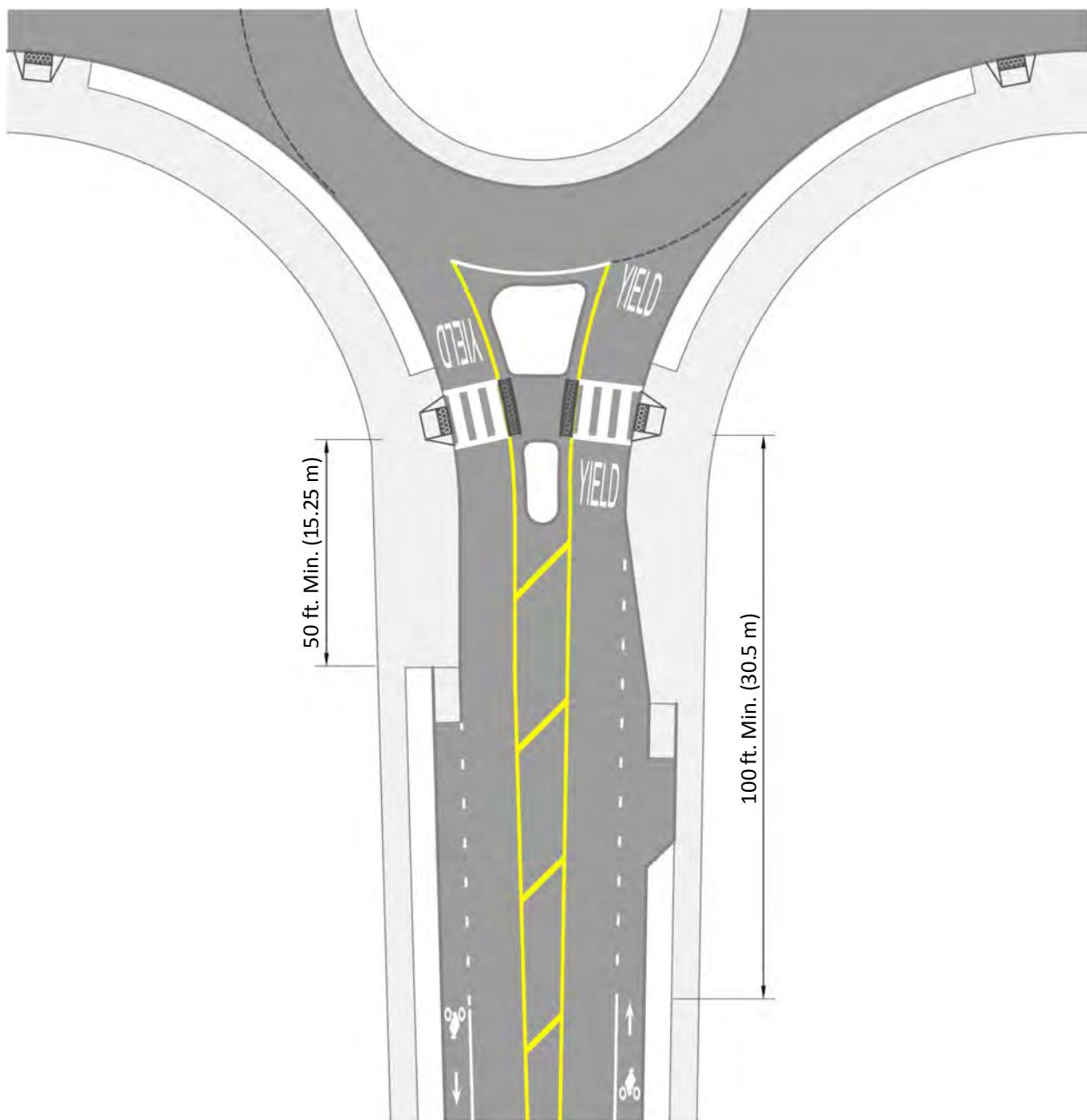
**Exhibit 4.43. Typical Layout of Roundabout with Bike Lanes (note: replace this drawing with new graphic based on final graphic proposed in the next edition of the FHWA Roundabout Guide – per Kittelson Assoc.)**
