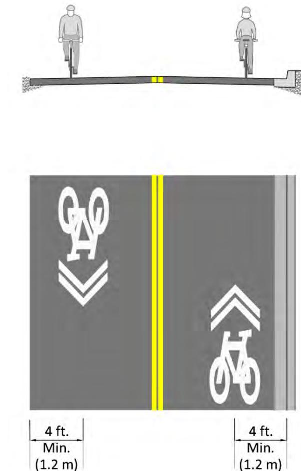
*Exhibit 4.6. Typical Shared Lane Marking Cross Section on Street with No On-Street Parking*
