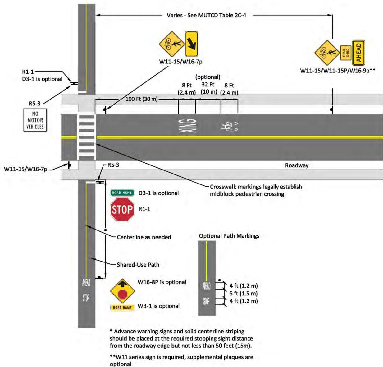
Exhibit 5.19. Example of Midblock Path-Roadway Intersection – Path is STOP Controlled
