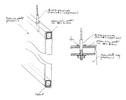
**Fig. 5.6** The double projection screen consists of two sides of semi-transparent white tectile material arranged in parallel to each other and organized in the same frame, which is lightweight enough to hang from two metallic threads; thus it looks like it is hovering
