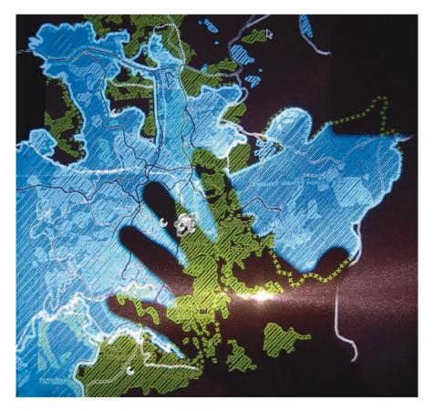
Fig. 5.4 In a double semi-transparent projection screen, if somebody blocks the image of one side, then the image of the other side is revealed
