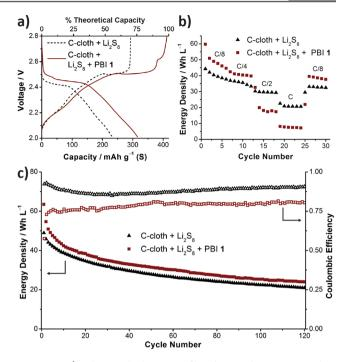
**Figure 4.** a) Charge—discharge profiles from galvanostatic cycling (second cycle) at a C/8 rate showing a 31% increase in discharge capacity for C-cloth +  $\text{Li}_2\text{S}_8$  + PBI 1. b) Rate performance at C/8, C/4, C/2, and 1C. c) Energy density (solid) and Coulombic efficiency (hollow)  $\nu s$ . cycle number at C/4 rate.
