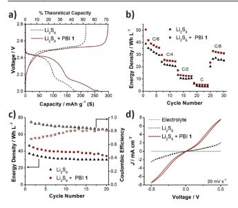
**Figure 3.** a) Charge—discharge profiles from galvanostatic cycling (second cycle) at a C/8 rate showing a 38% increase in discharge capacity for PBI  $1 + \text{Li}_2S_8$ . b) Rate performance at C/8, C/4, C/2, and 1C. c) Energy density (solid) and Coulombic efficiency (hollow) vs. cycle number at C/8 rate. d) IV curves from cyclic voltammetry with an interdigitated array electrode.
