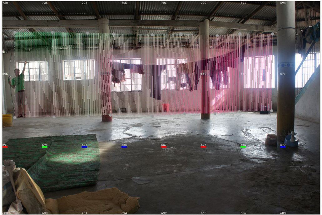
Figure 2 Tippu Tip House 2nd level. Visualization shows a lot of cross ventilation close to the windows.
