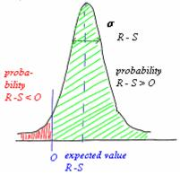
Figure 2: Statistical test for R - S
