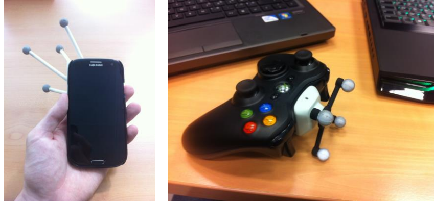
Figure 2 : The peripheral used for the experiment with a body of tracking: a Samsung Galaxy SIII (left) and an XBOX 360 gamepad (right)
