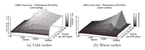
Fig. 3. IP performance, using N/P reduction. Working set: 16×#psize bytes.
